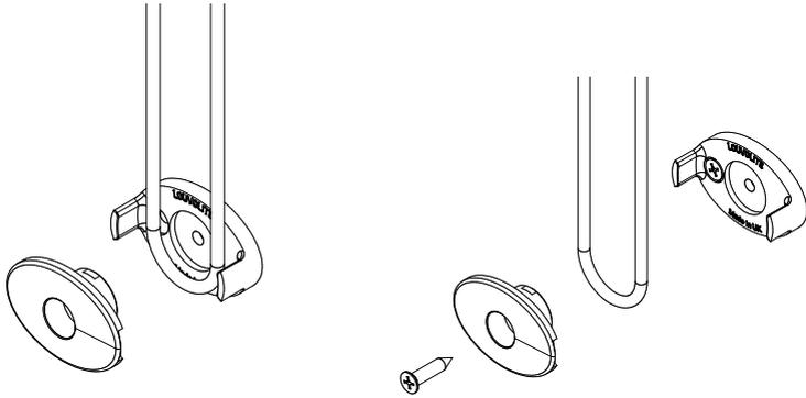
Push fit a cover cap over the screw hole opening.
