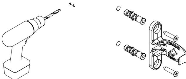
Attach the cord cover plate with the screw provided.
