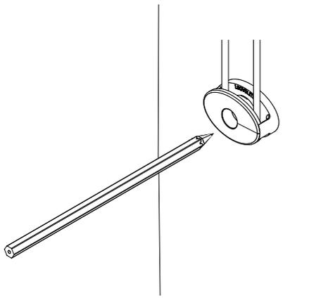
Split the cord tidy and mark the remaining offset hole position before drilling and plugging both location holes if necessary. Screw into the offset hole to fix the back piece of the cord tidy to the wall.
