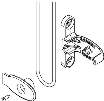
Push fit a cover cap over the screw hole opening.
