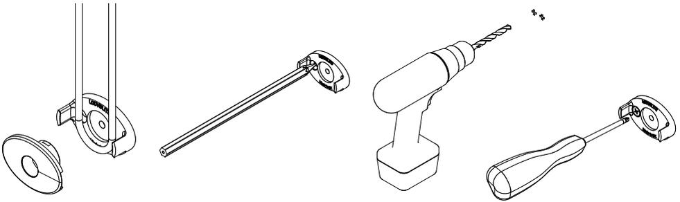
Re-assemble the cord tidy with the cord and fix it in previously marked position with a screw through the centre hole.
