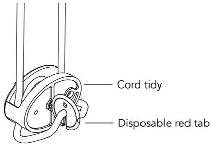
Remove the disposable red tab by disengaging it from the cord and then pull out the disposable red tab.
