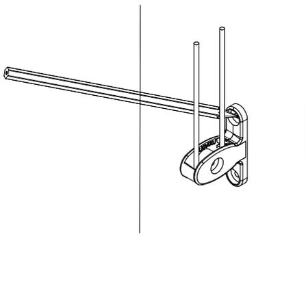
Mark the remaining hole position before drilling and plugging both location holes if necessary.
